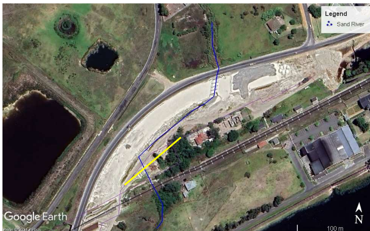
Figure 22: Watercourse delineation Map for the Sand River at the proposed sewerage pipeline crossing point. The blue line indicates the alignment of the Sand River and the yellow line the approximate position of the proposed sewerage pipeline. Note the extent of earthworks immediately south of the R310.
