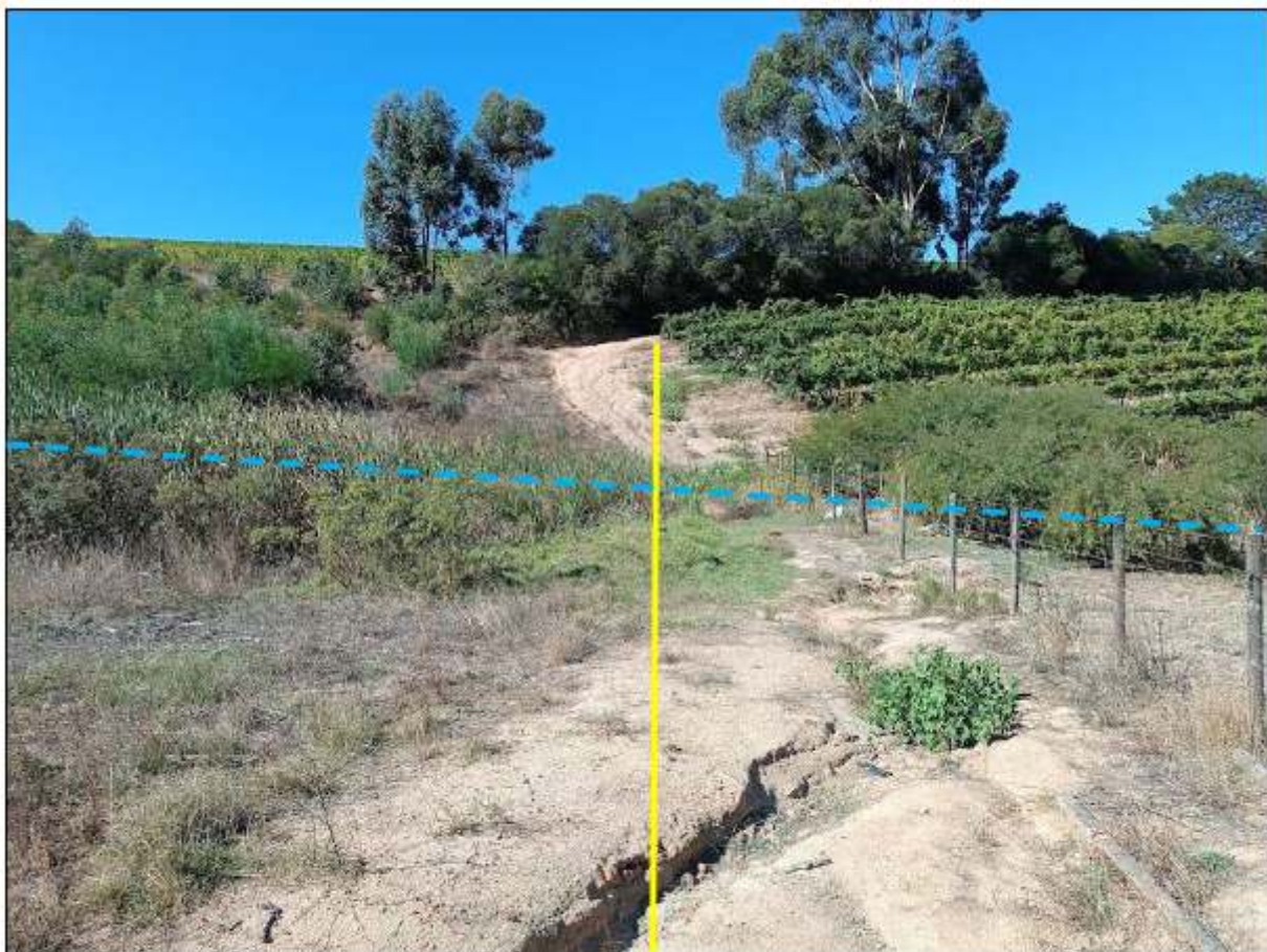
Figure 12: Photograph of the proposed water pipeline crossing of the 'clean' watercourse. The approximate alignment of the pipeline is indicated as a yellow line and the watercourse as a blue stippled line. Note the erosion of the farm road in the foreground
